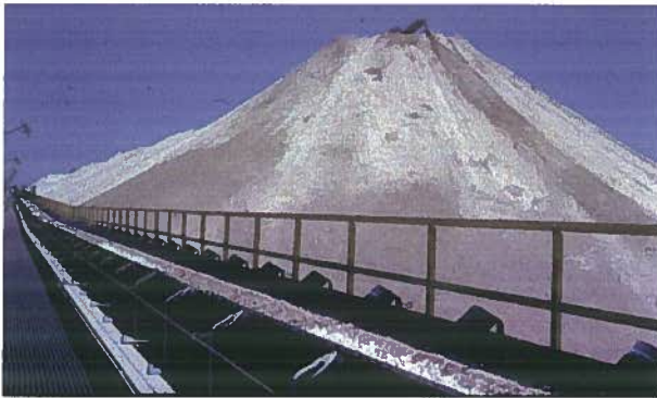
Fig 8 (a) Dry transport to stack in valley; (b) Settlement cracks in dry stack in valley
