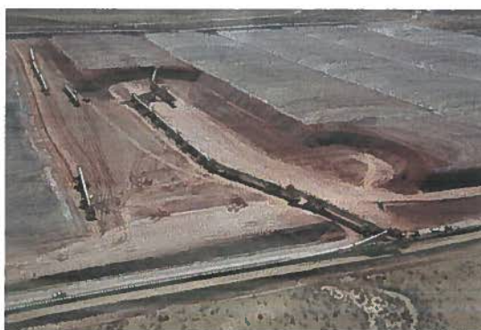
Fig 11. Self-contained movable spreader/stacker
