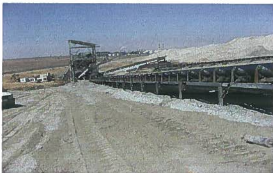
Fig 7. (a) Dry transport by conveyor belts; (b) Dry transport by trucks
