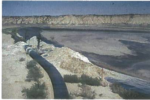
Fig 5. Gypsum slurry deposition using spigots
