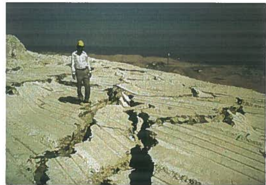
Fig 8 (a) Dry transport to stack in valley; (b) Settlement cracks in dry stack in valley
